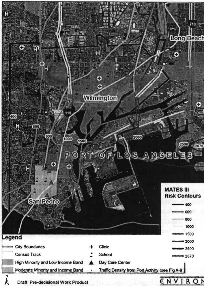
Figure 12. DPM residential cancer risk from the 2005 modified MATES III simulation, overlaid on the background map of the Port region and including all sensitive receptors identified in this analysis. (A full-size version of this figure is presented in Appendix A as Figure A-12.)
