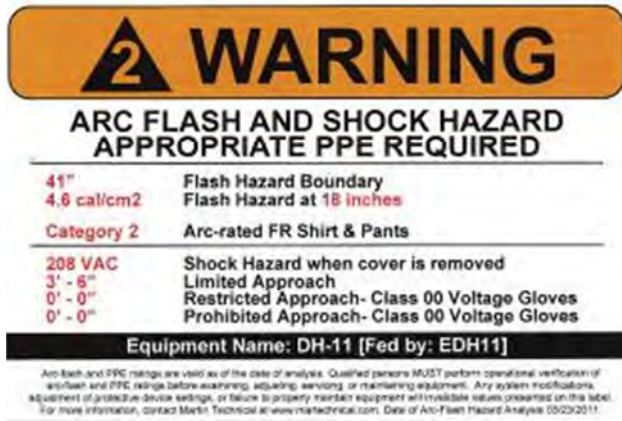
Sample Arc Flash Label from Arc Flash Analysis
