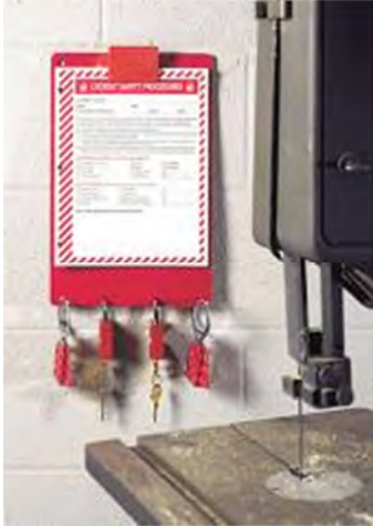
Examples of wall mounted Lockout / Tagout stations for procedures.
