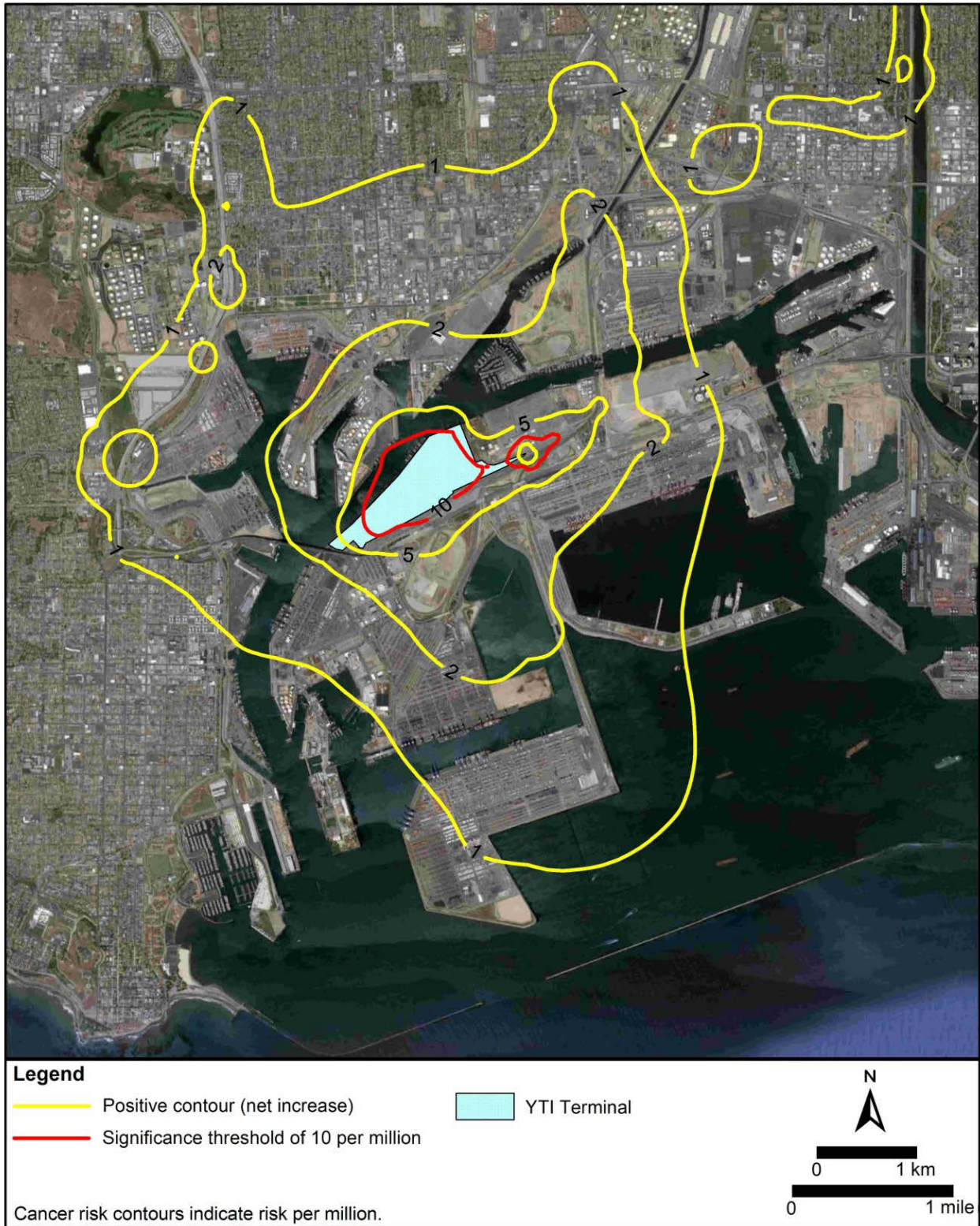
Figure 7-15. Isopleths of Residential Lifetime Cancer Risk: Proposed Project without Mitigation Minus NEPA Baseline
