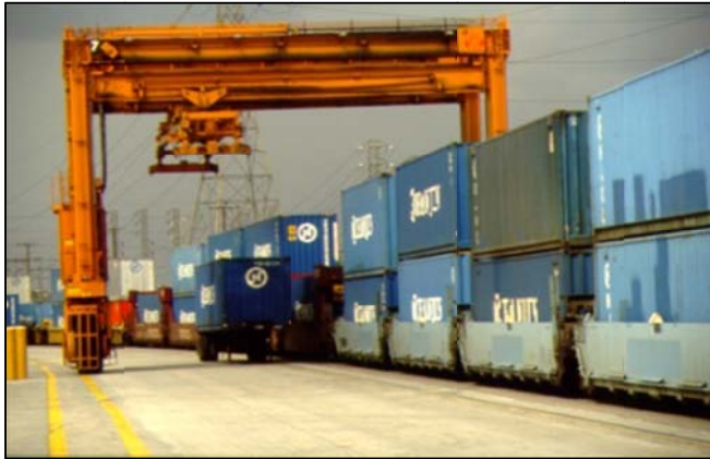
1 Figure 1-9. General Depiction of Train Loading/Unloading at an Intermodal Railyard.
