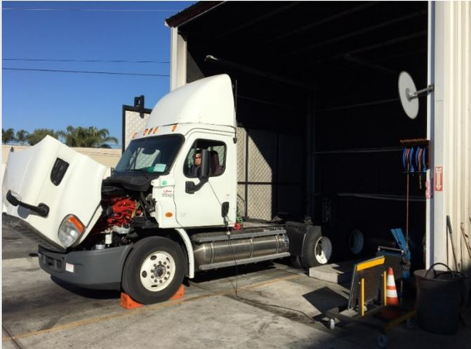
Dynamometer Test of TTSI Truck
