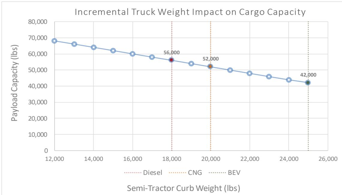
Figure 10. Incremental truck weight impacts on cargo capacity
