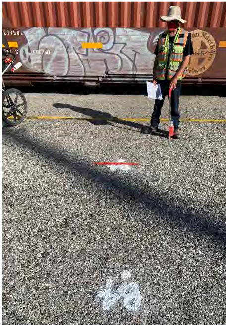
Photograph 1: Geophysical survey at Boring B4 identifying electrical line which required relocation of boring B4.
