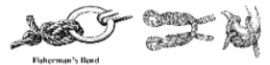
Fisherman's Bend: A good line to have a fish on the line is a fisherman's bend. It is used for securing the line to a hook.
