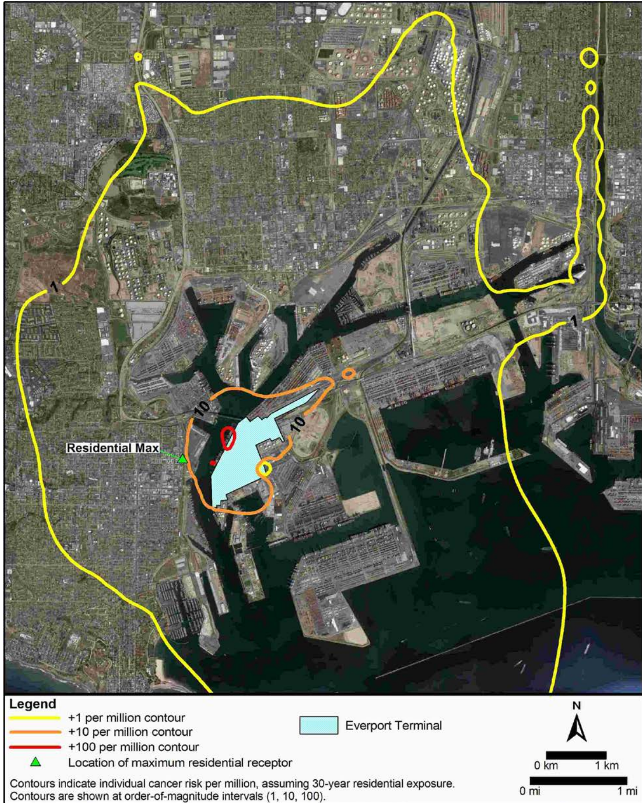
Figure B3-8: Isopleths of 30-Year Residential Cancer Risk – Proposed Project with Mitigation – NEPA Increment
