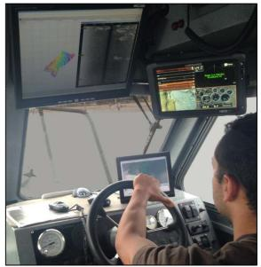
Survey vessel used to map eelgrass and provide bathymetric and sidescan waterfall data.
