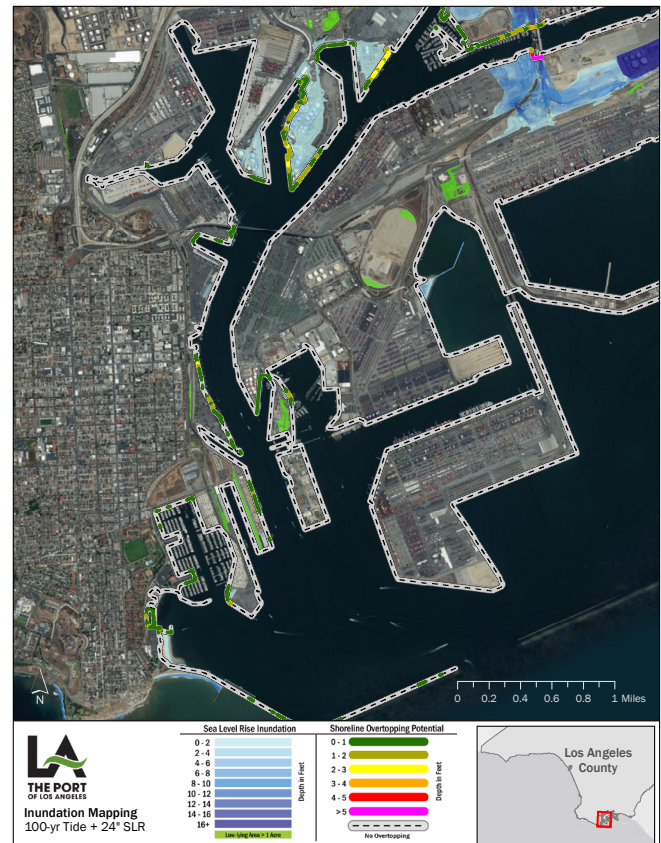
Figure 4-3. Example flooding and inundation map
