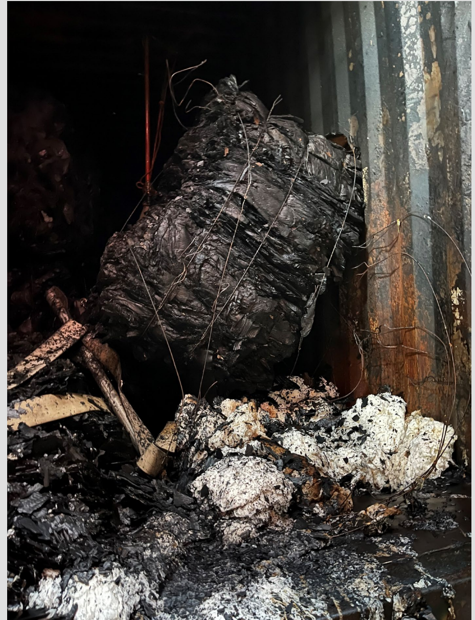
Above: Container full of cotton that had been a source for reflash; now considered wet cargo
