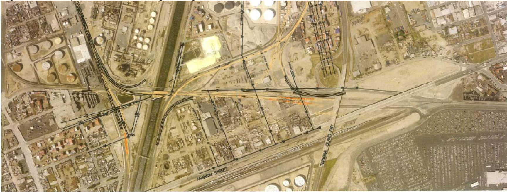
1 Figure 3.11-2. Proposed Site Plan Showing Existing Utilities and the Relocation Site Areas.
