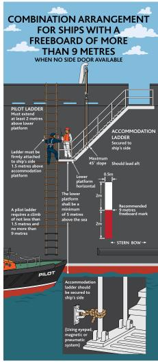
NOTE: - The pilot ladder is required to be rigged two (2) meters above the water.
