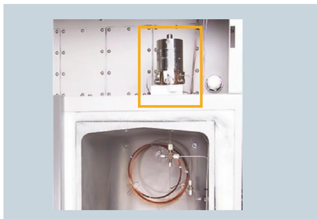
Fig. 6 Flame Ionization Detector combined with a capillary columns set in an airless oven
