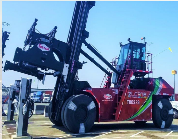
Taylor - Battery Electric New Build with plug-in charging at EverPort
