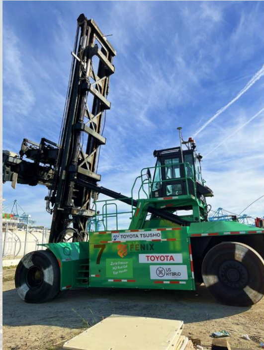
Toyota Tsusho - Hydrogen Fuel cell repower at Fenix
