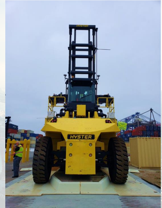
Hyster - Battery Electric with Hydrogen Range Extender New Build with inductive charging at Fenix
