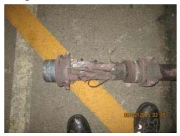
Forward cable plug housing completely damaged and burnt off
