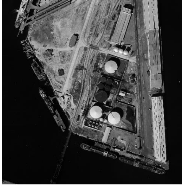
Figure 46: Berths 150-151 as it appeared in 1939: one marine oil terminal, approximately sixteen tanks in tank farm, original office and warehouse present, compacted dirt surfaces, access roads; wharf at Berth 149 added, wharf at Berths 150-151 extended. USCB Library.
