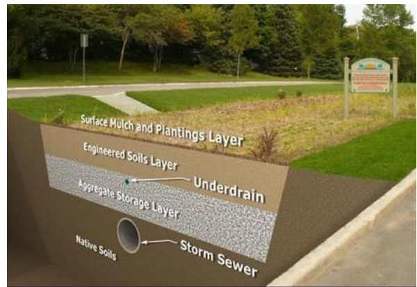
Figure 2. Bioretention Swale Cross Section
