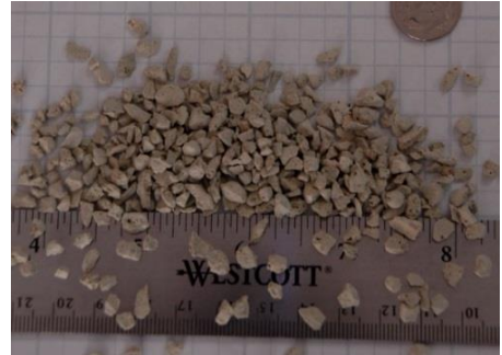
Figure 5. KMI Zeolite (4x8 size) - currently utilized at the New Dock Pump Station
