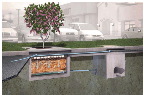
Figure 4. Standard Filterra® System with Curb Inlet
