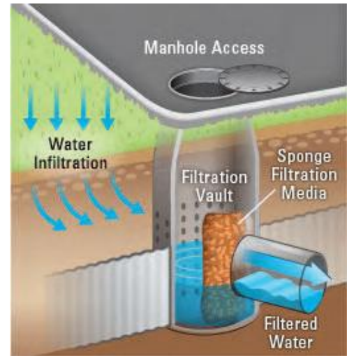
Figure 9. MetalZorb® installed in a filtration vault
