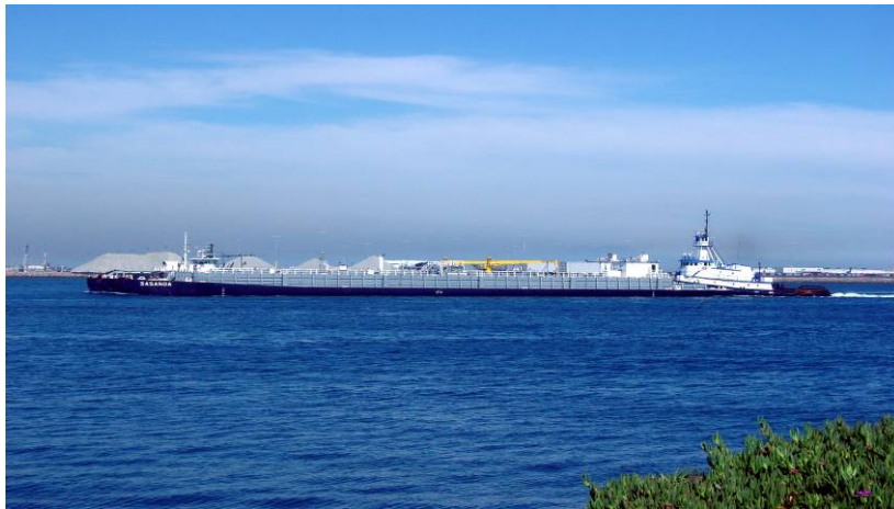
Figure 2.11: Integrated Tug and Barge
