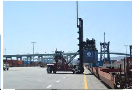
Containers loaded/unloaded to train cars at on-dock railyard
