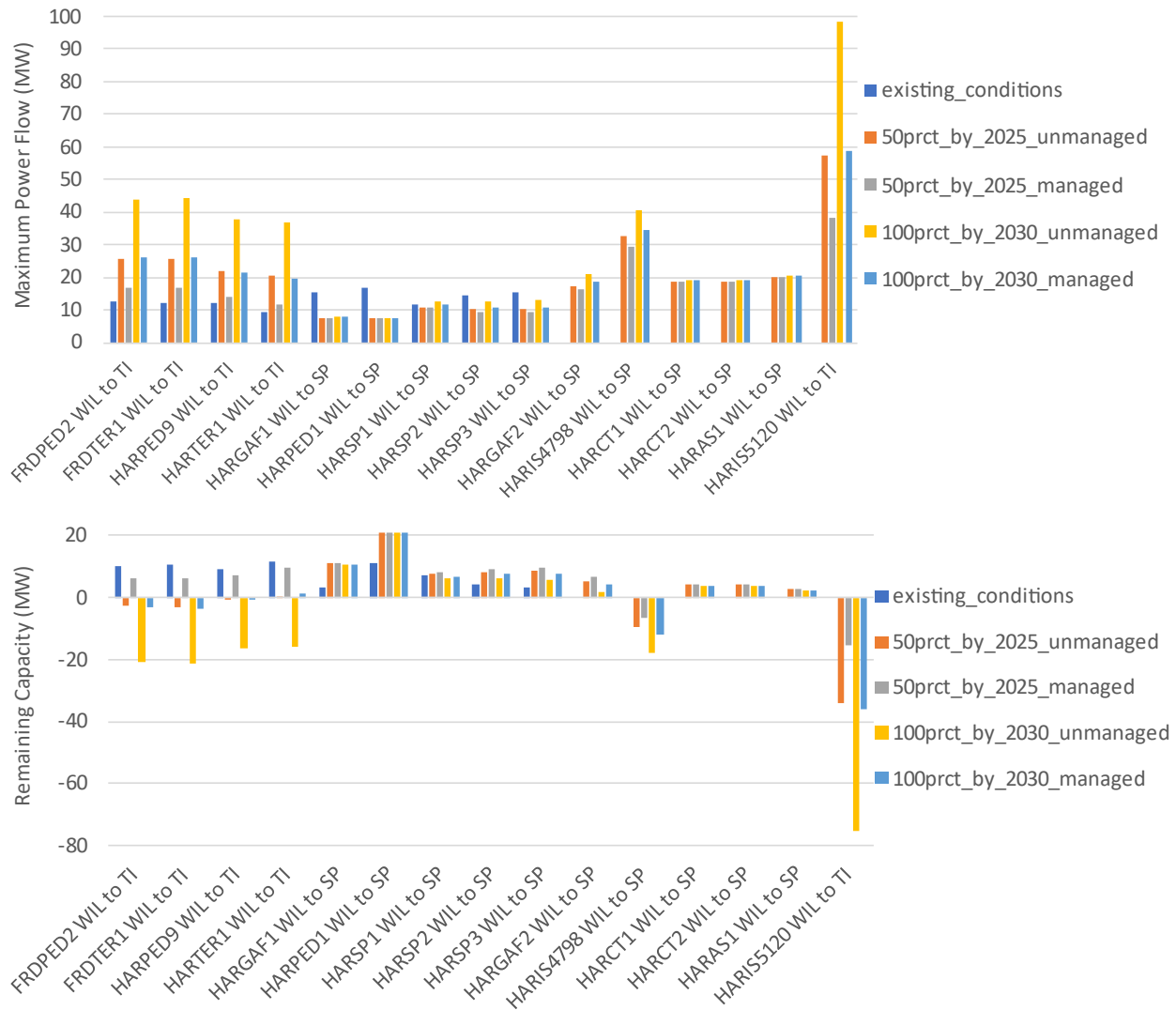
Figure 43. Maximum power flows (top) and remaining capacity (bottom) on the tie-lines at the area boundaries—future lines planned by LADWP included
