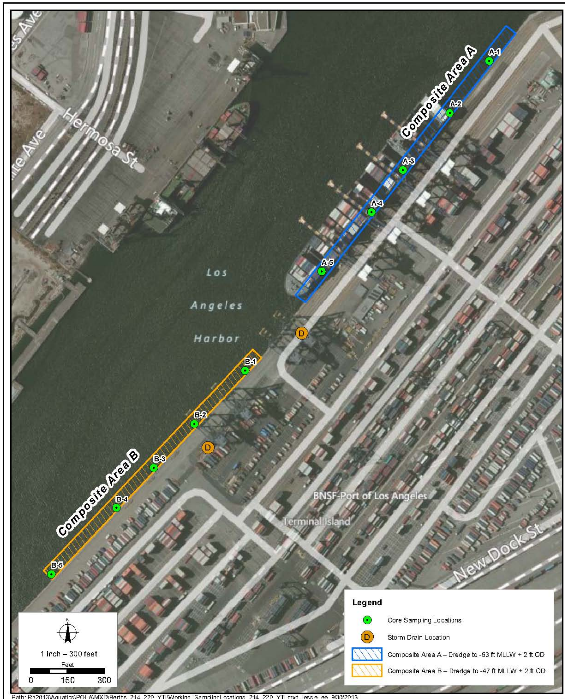
amec Core Sampling Locations Berths 212-224 [YTI] Container Terminal Improvements Project Port of Los Angeles FIGURE 2-1
