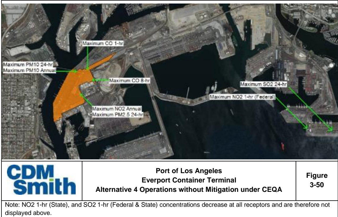
Figure 3-50. Maximum Air Quality Impact Locations – Alternative 4 Operations without Mitigation under CEQA
