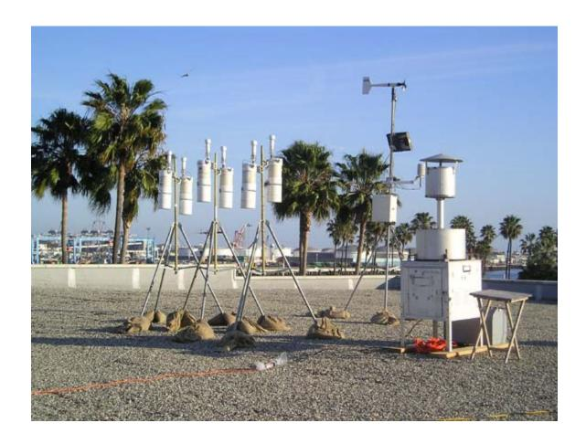
Under a proposed agreement between the ports of Los Angeles and Long Beach, a network of air quality monitoring stations similar to the one pictured here will provide real-time air quality monitoring in and around the port complex.
