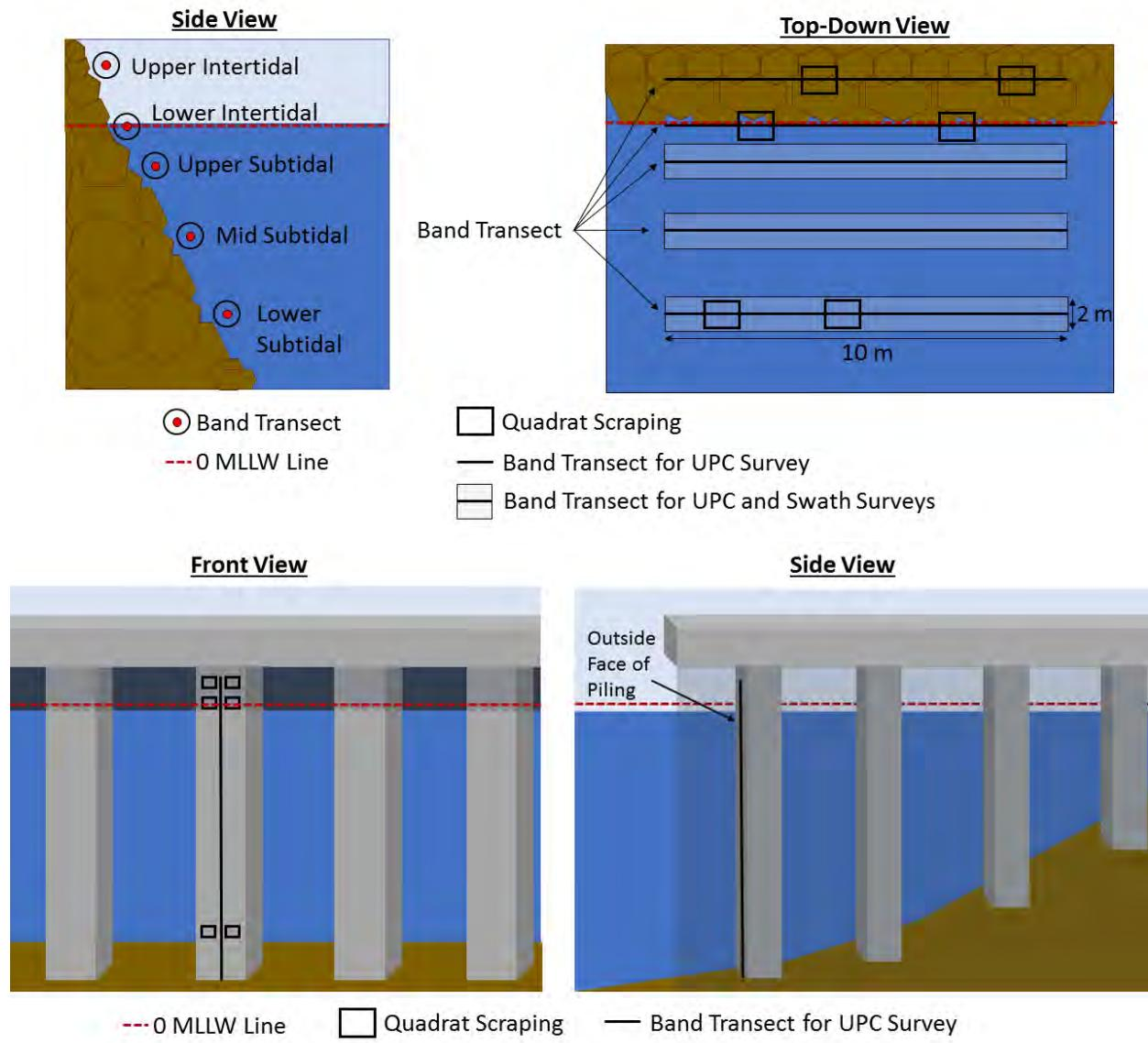
**Figure 5-8. Riprap and Concrete Pier Piling Scraping Site Schematic**
