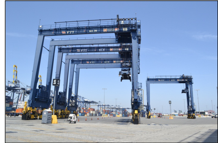
Photograph 3: Rubber-Tired Gantry (RTG) Cranes
