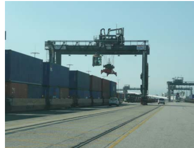
Containers loaded/unloaded to train cars at on-dock railyard
