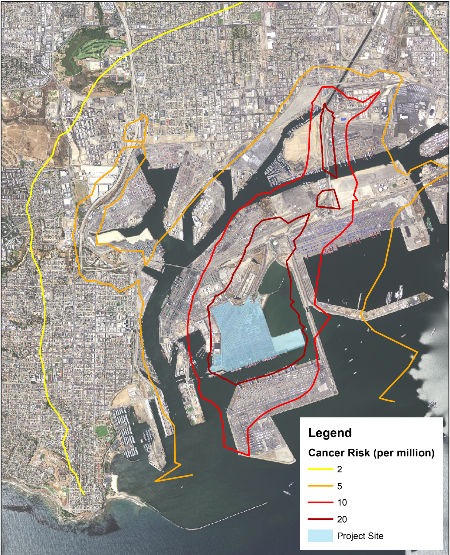
Port of Los Angeles Berths 302 - 306 [APL] Container Terminal Project Isoleths of Residential Lifetime Cancer Risk: Mitigated Proposed Project Minus Future CEQA Baseline
