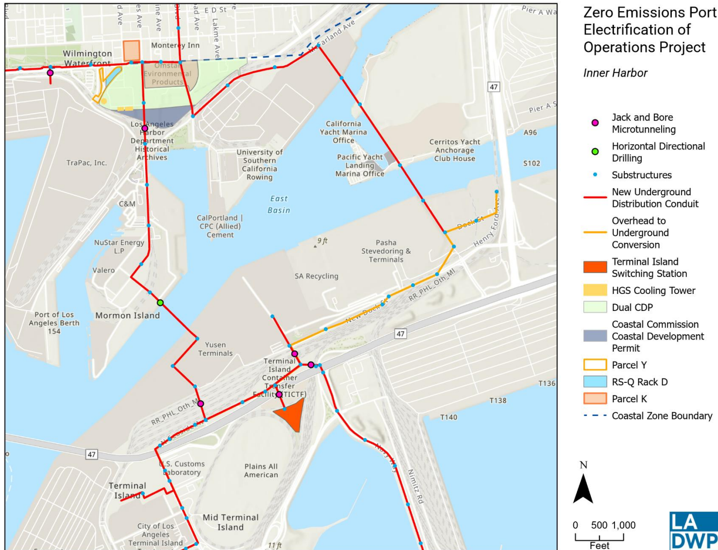
Figure 1-5 New Underground Distribution and Overhead to Underground Distribution Conversion Locations Within the Inner Harbor
