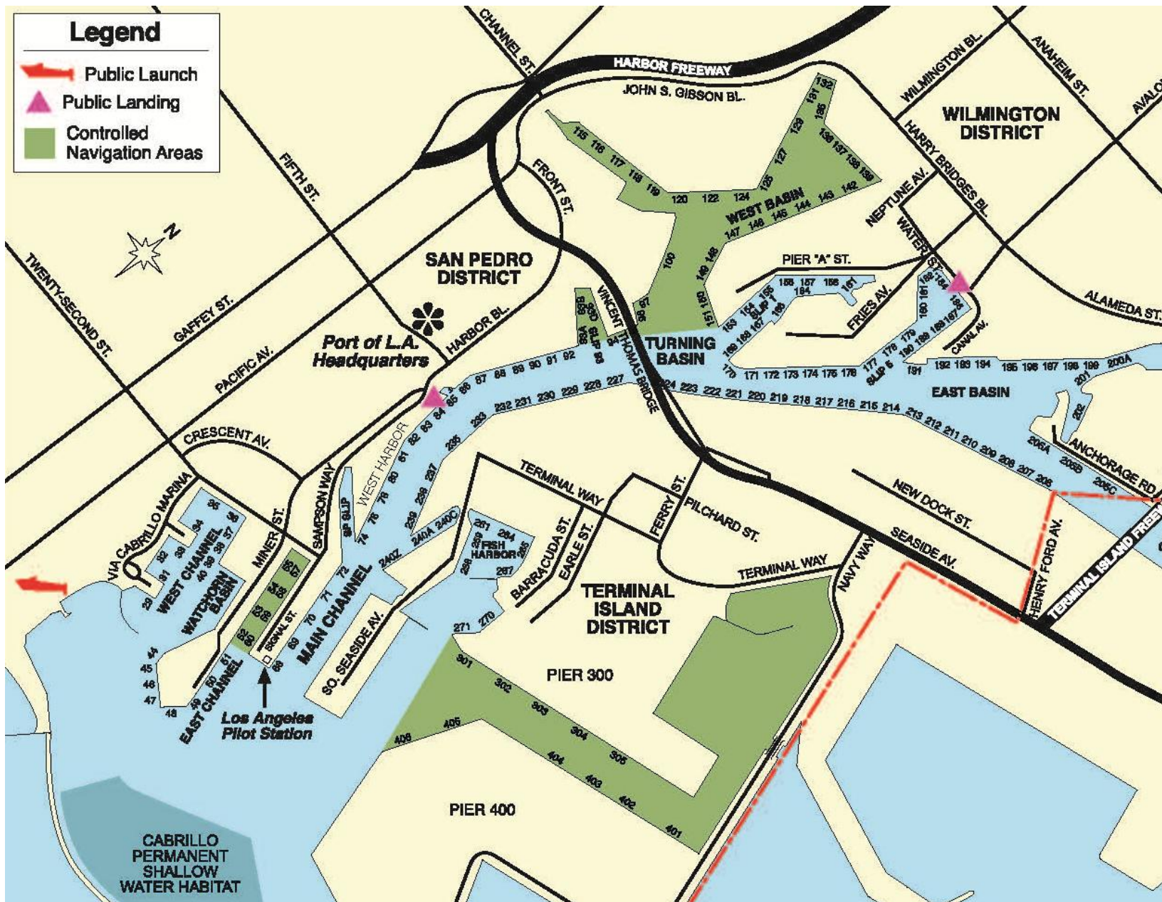
Figure 1-10 Navigational Descriptions for the Port of Los Angeles Including Berth Numbers, Channel Names, and Basin Names
