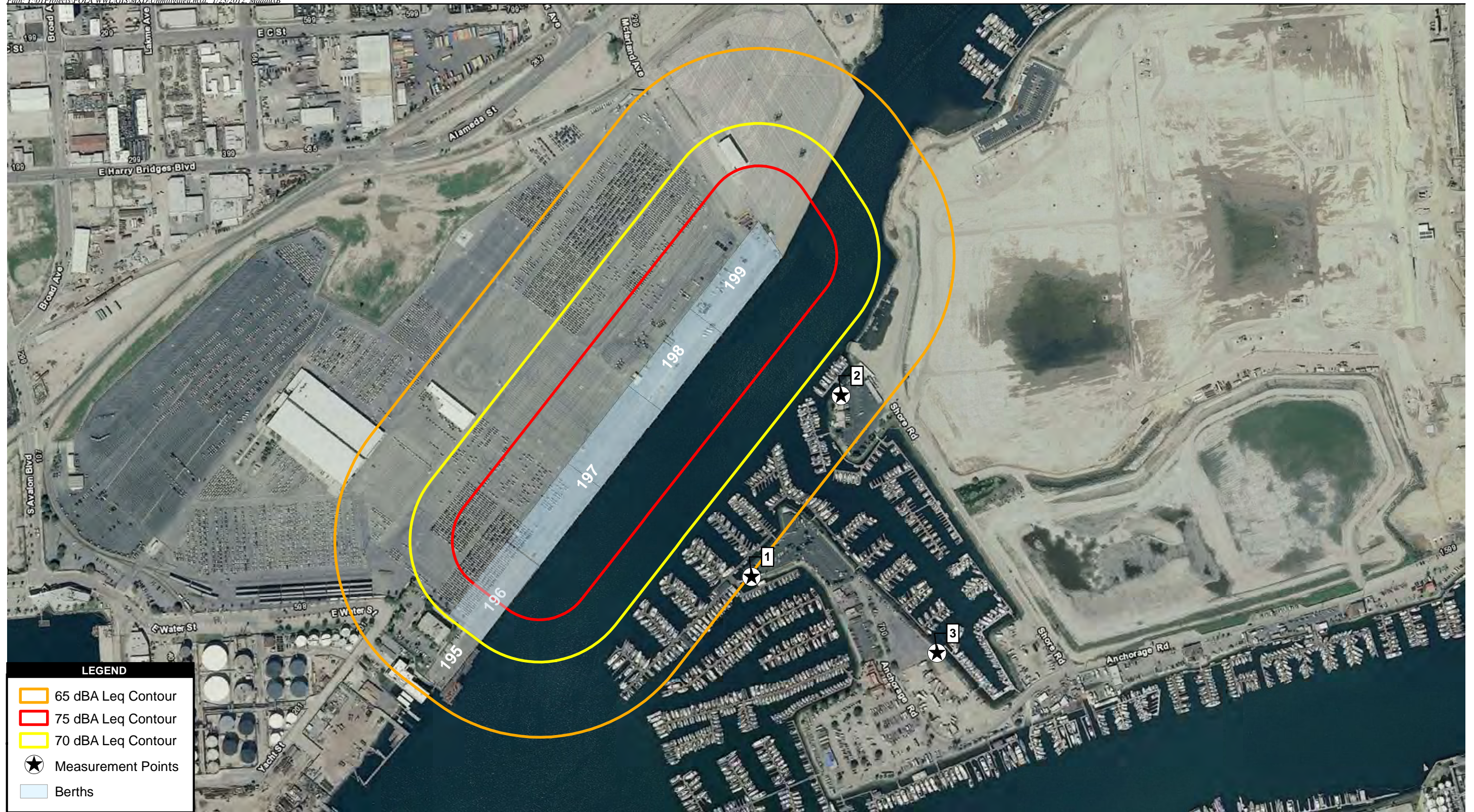
Figure 4.12-1 Unmitigated Pile Driving Noise Contours
