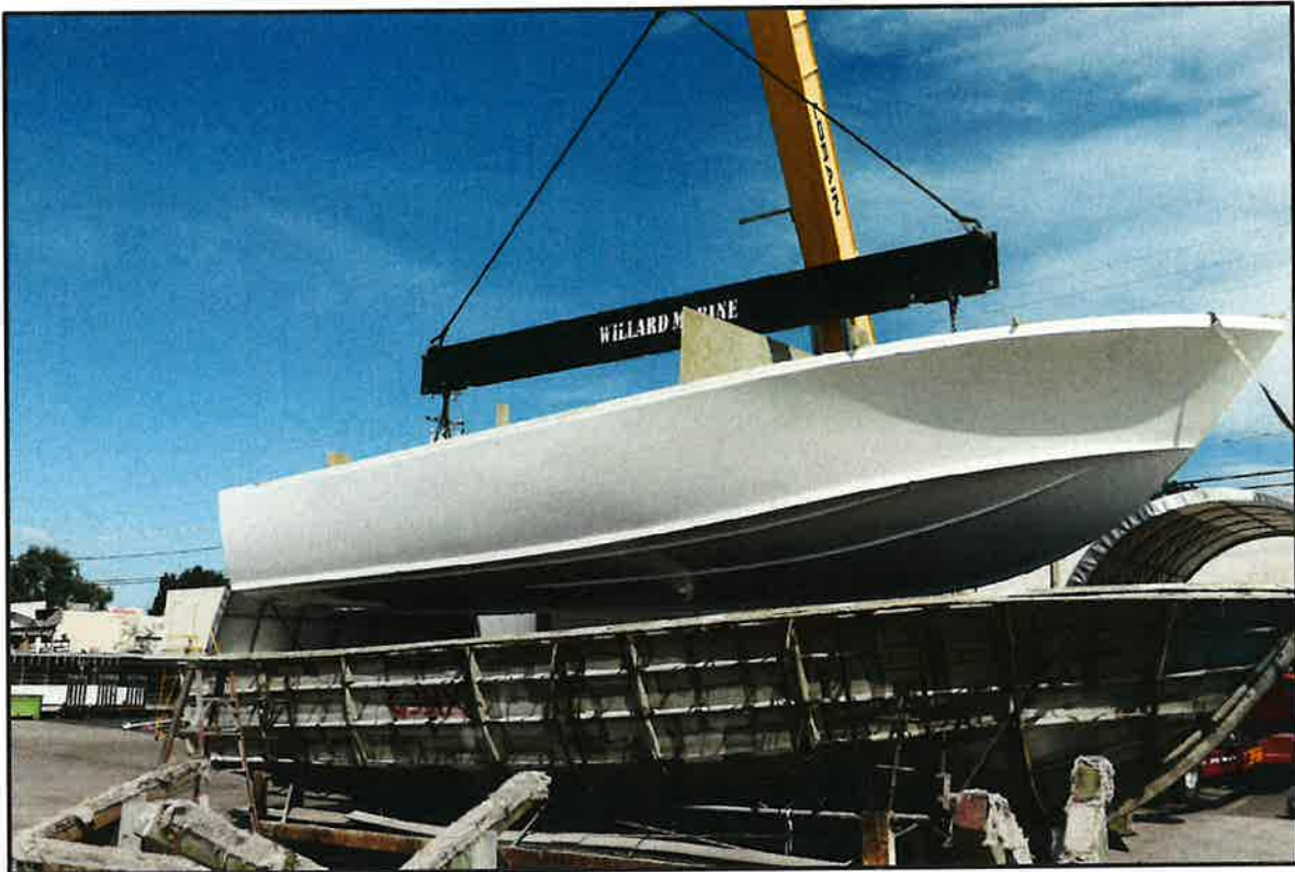
Figure 9: QA & Testing: Pulling Hull out of the Mold
