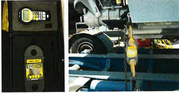
Figure 7: Dynamometer load testing equipment
