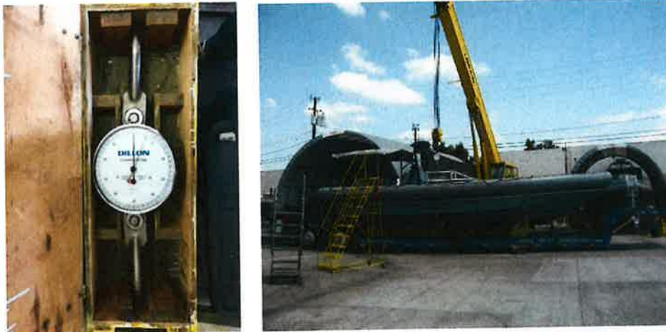
Figure 6: Willard Marine overload testing during 11MRB contract
