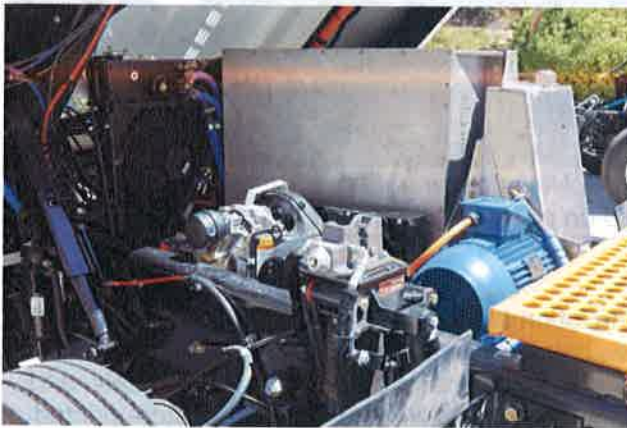
Figure 15. Single ICU PCAS assembly installed in second generation prototype electric yard tractor.
