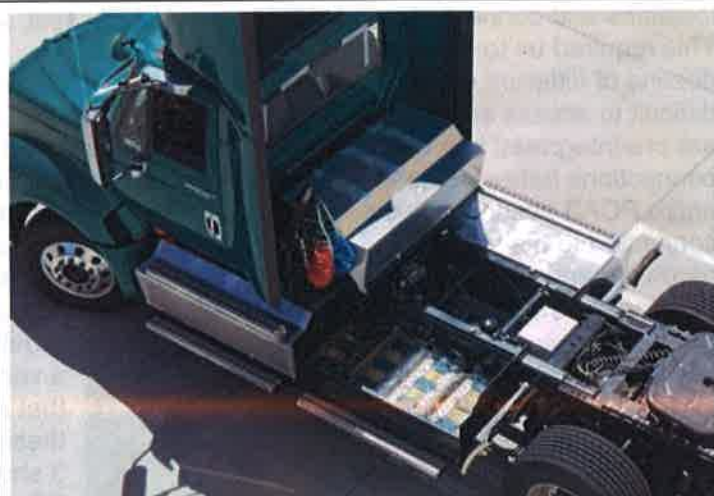
Figure 13. New design battery enclosures – only 3-5 required on each Class 8 drayage truck or yard tractor.
