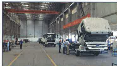
BYD YARD TRACTOR ASSEMBLY LINE
