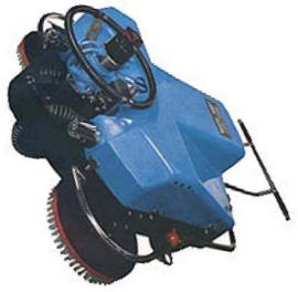
Hydraulic triple brush "Scamping" machine used for large ship surfaces.
