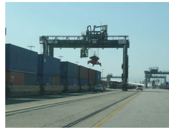
Containers loaded/unloaded to train cars at on-dock railyard
