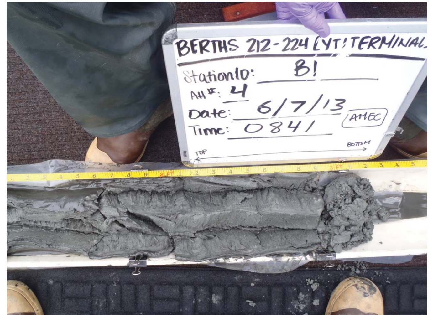
Location: POLA Berths 212 - 224 (YTI Terminal) Sample ID: B1 Attempt #: 4 Core Length: 1.0 - 3.3 ft. Sample Date & Time: 06/07/2013 0841
