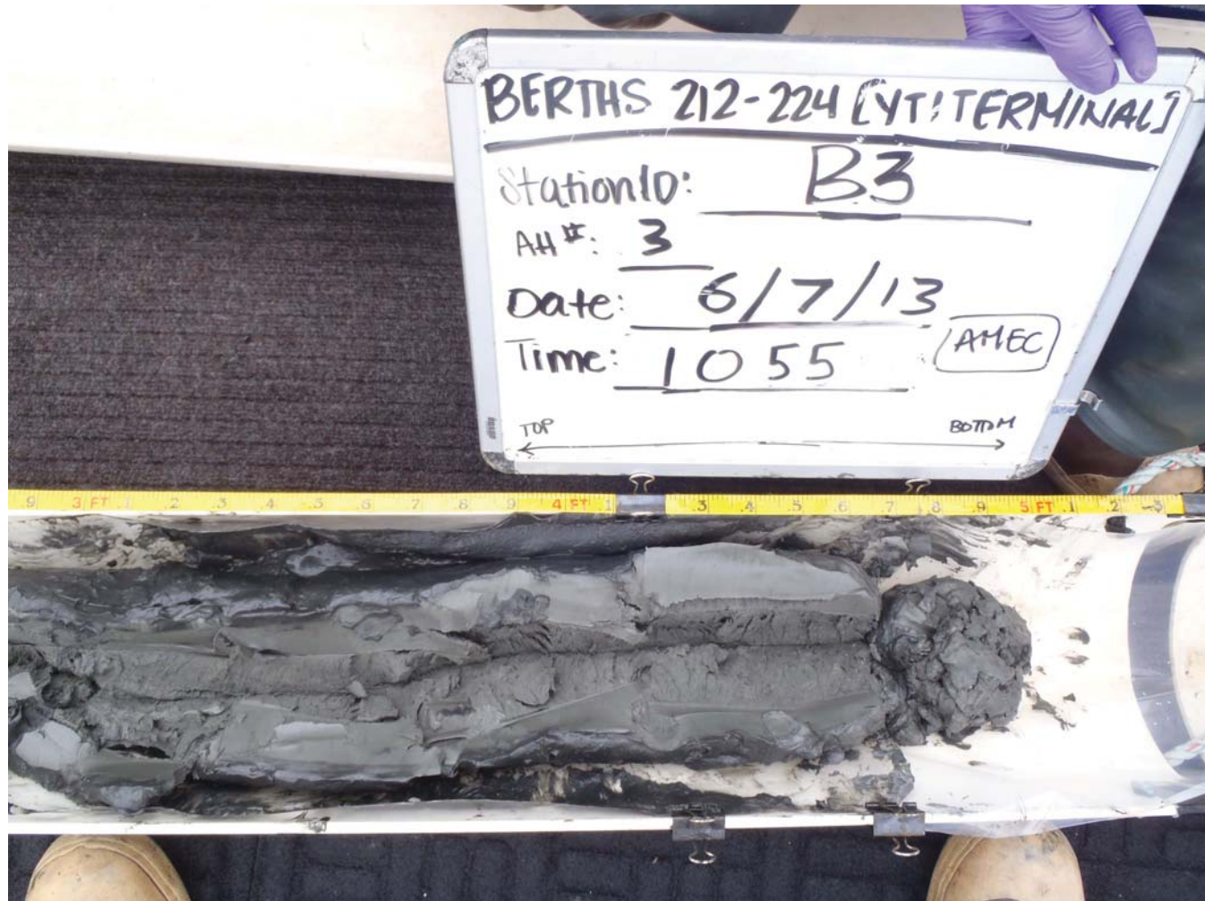
Location: POLA Berths 212 - 224 (YTI Terminal) Sample ID: B3 Attempt #: 3 Core Length: 3.0 - 5.0 ft. Sample Date & Time: 06/07/2013 1055
