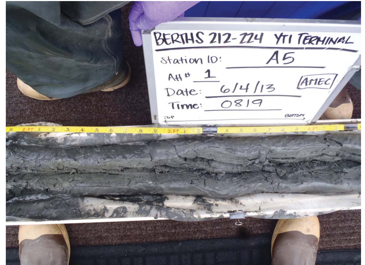
Location: POLA Berths 212 - 224 (YTI Terminal) Sample ID: A5 Attempt #: 1 Core Length: 2.0 - 4.0 ft. Sample Date & Time: 06/04/2013 0819
