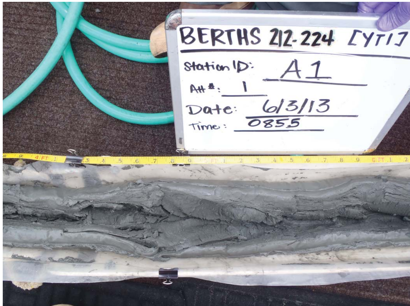
Location: POLA Berths 212 - 224 (YTI Terminal) Sample ID: A1 Attempt #: 1 Core Length: 4.0 - 6.0 ft. Sample Date & Time: 06/03/2013 0855
