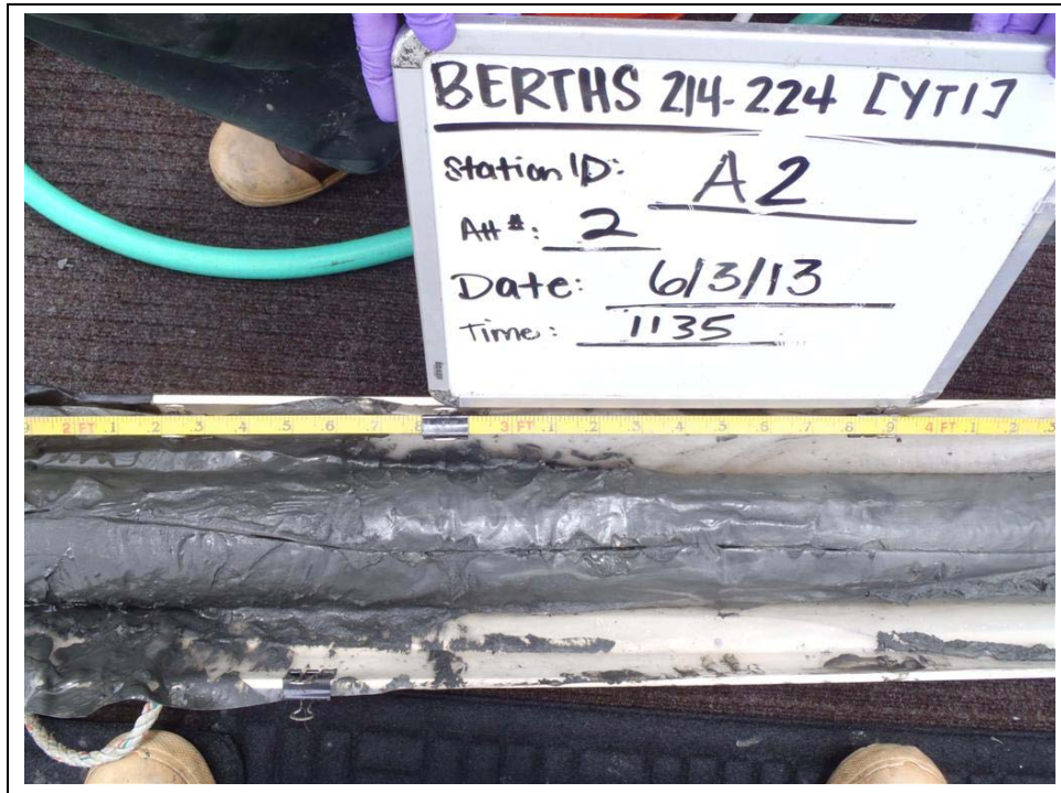
Figure 4-2. Transition from Silt to Clay Sediment (2–4 ft below harbor bottom)
