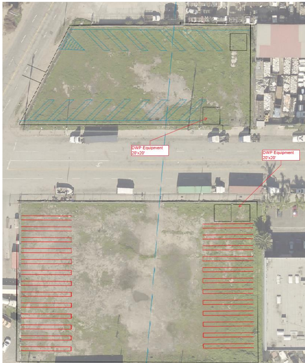
Figure 4. Conceptual site layout for the public access charging facility
