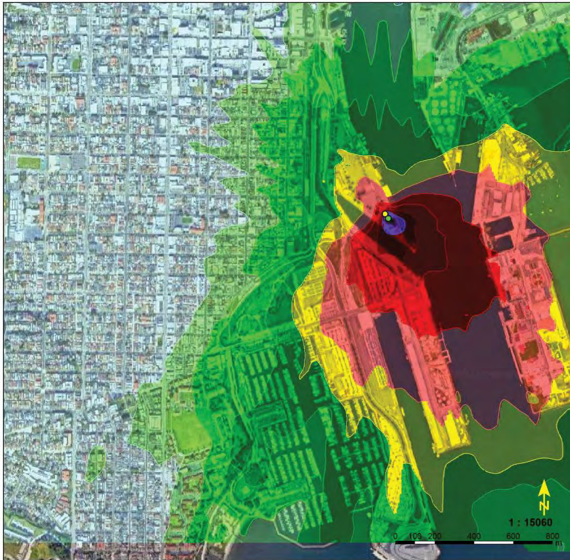
Figure 3.8-3 Noise Contour Maps of Community Noise Levels at 16-foot Elevation, from Amphitheater with Favorable Atmospheric Conditions West Harbor Modification Project
