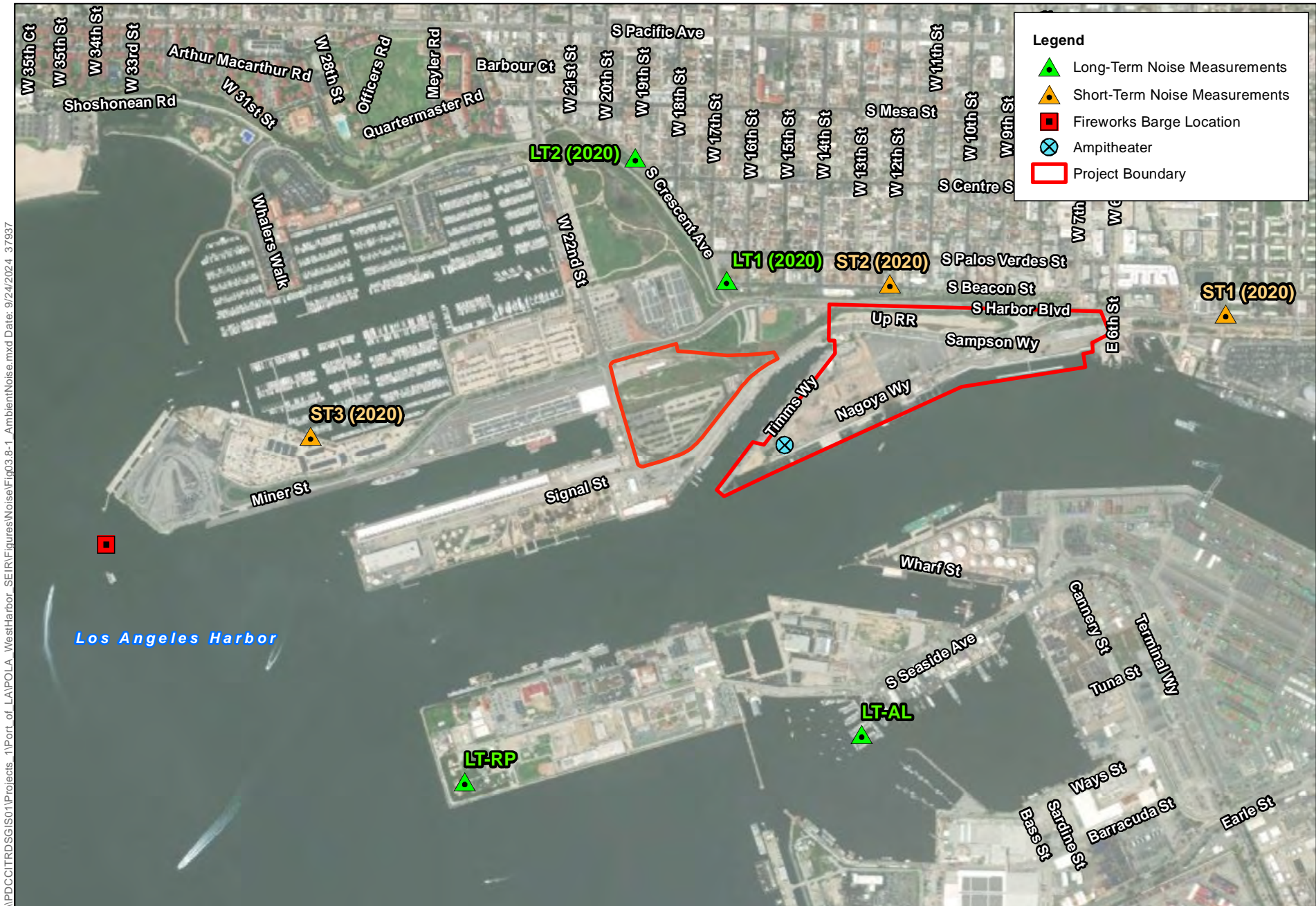
Figure 3.8-1 Ambient Noise Measurement Locations West Harbor Modification Project
