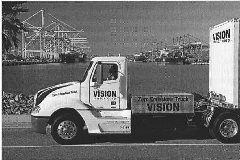
Figure 2 Vision Zero-Emission Fuel Cell Battery Electric Truck
