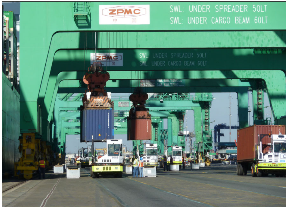
Photograph 2-6: Container being loaded onto yard tractors at the wharf.
