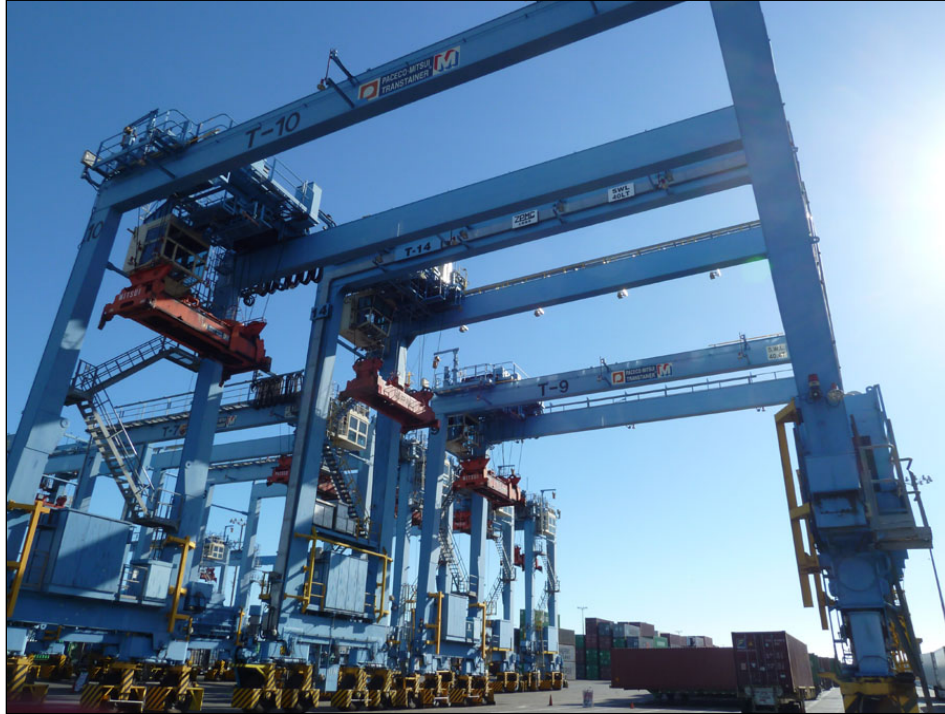
Photograph 2-10: Rubber Tired Gantry Crane (RTG).
