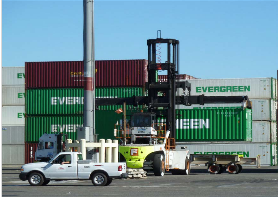
Photograph 2-7: Top handler loading a yard tractor.
