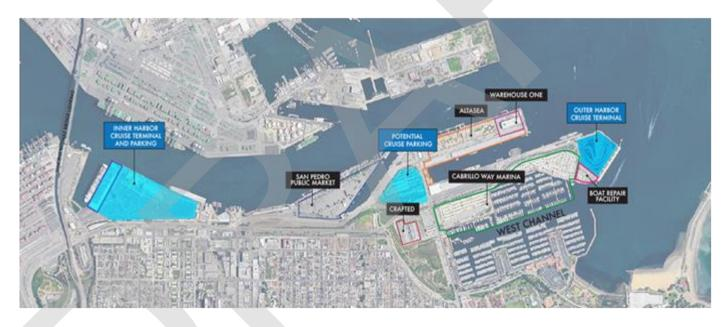
The Outer Harbor Cruise Terminal has two existing wharves, Berths 45-47 and Berths 49-51. Berths 45-47 feature a 900-foot concrete wharf with at-berth water depths exceeding 45 feet. Berths 49-51 have a 800-foot existing concrete wharf with minimum at-berth water depths of 35-45 feet. Berths 49-51 can potentially be extended up to 1,400 feet.
