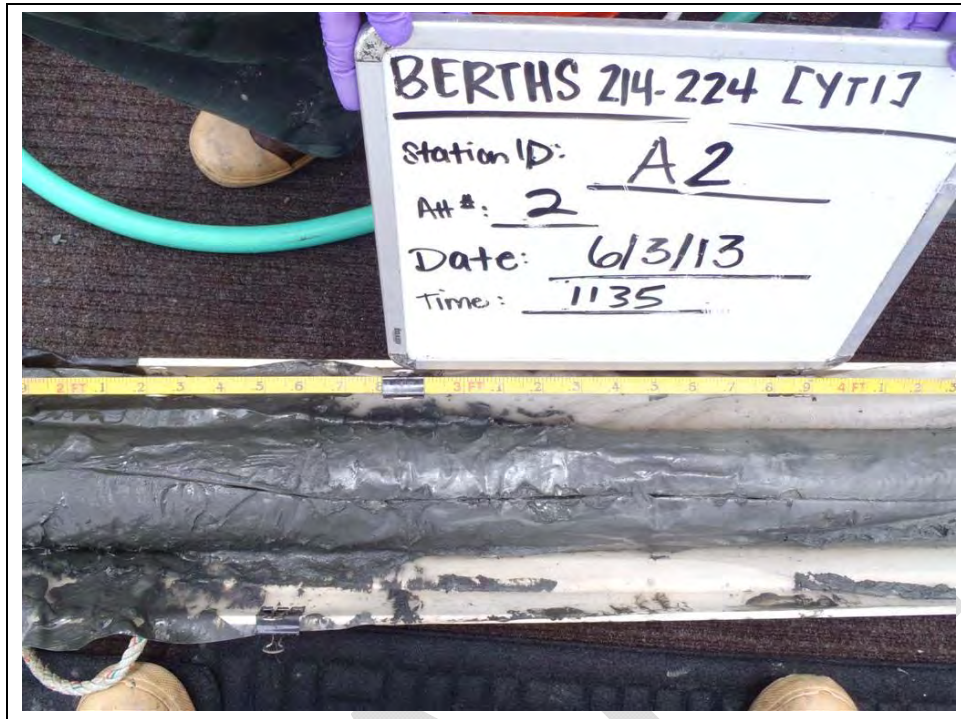
Figure 4-2. Transition from Silt to Clay Sediment (2–4 ft below the harbor bottom)
