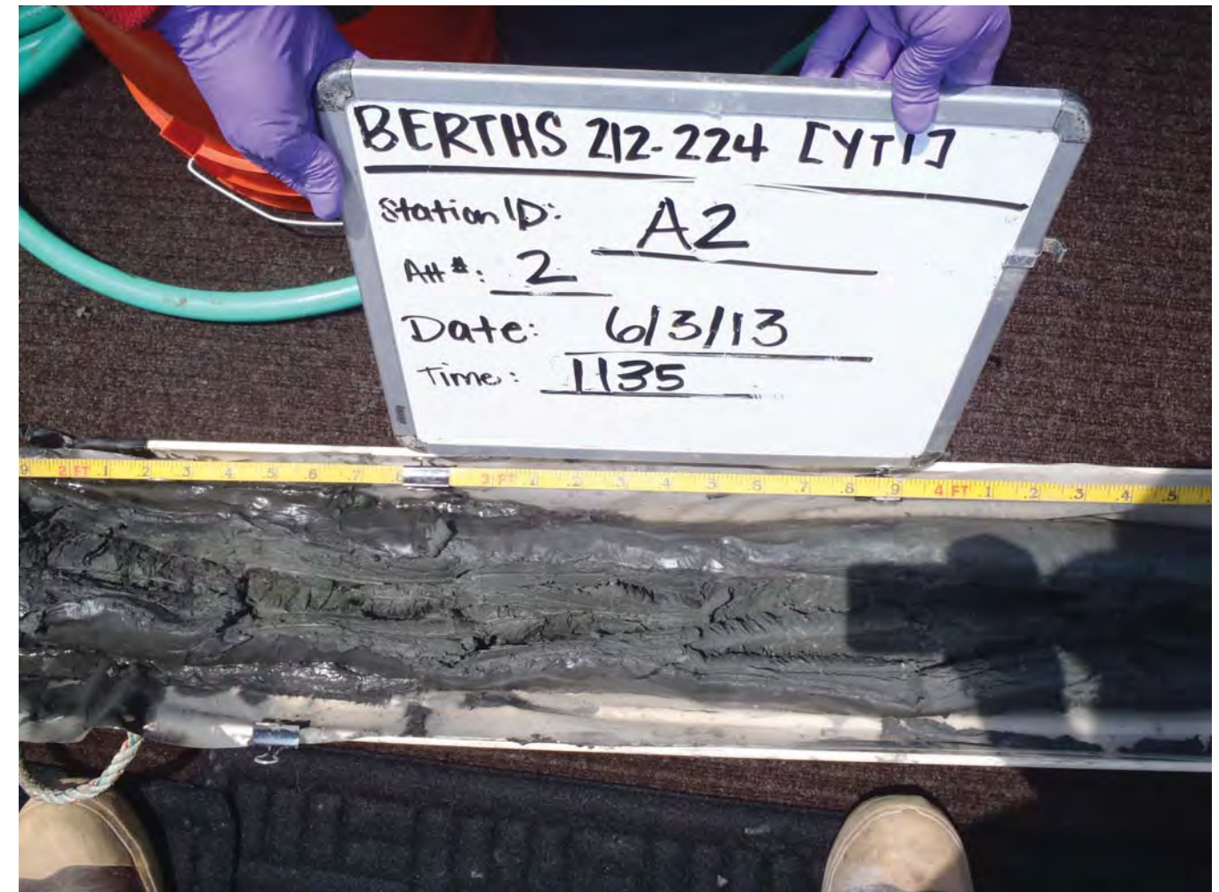
Location: POLA Berths 212 - 224 (YTI Terminal) Sample ID: A2 Attempt #: 2 Core Length: 2.0 - 4.0 ft. Sample Date & Time: 06/03/2013 1135
