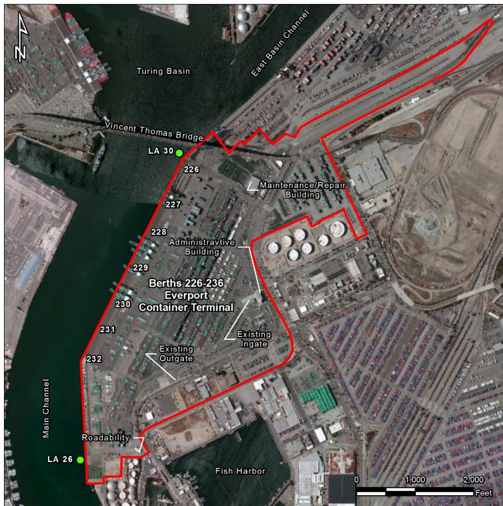
Figure 3.11-1: Location of proposed Project site and water quality stations LA 26 and LA 30
