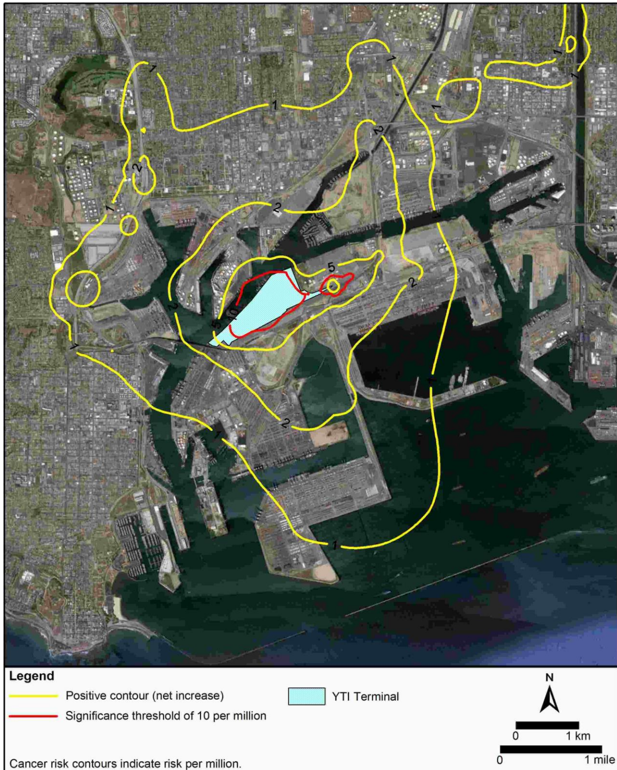
1 Figure 3.2-8: Isopleths of Residential Lifetime Cancer Risk: Unmitigated Proposed 2 Project Minus NEPA Baseline
