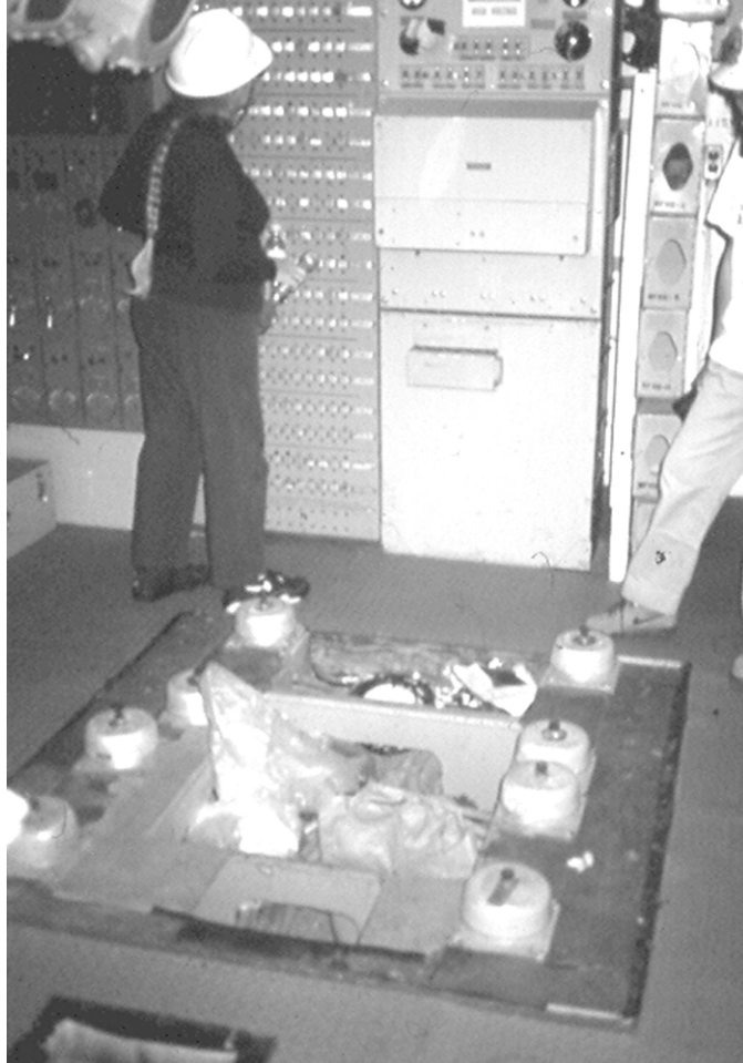
ONLY SHOCK MOUNTS LEFT OF MK-48 COMPUTER IN AFT MAIN BATTERY PLOT
