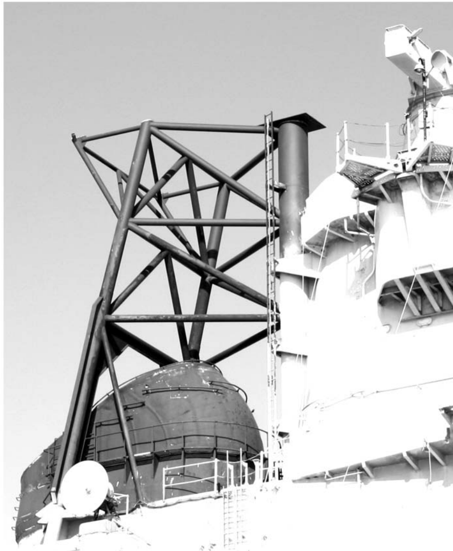
2006 PHOTO SHOWS MAST AS IT WAS CUT TO CLEAR A LOW BRIDGE TO BENICIA
