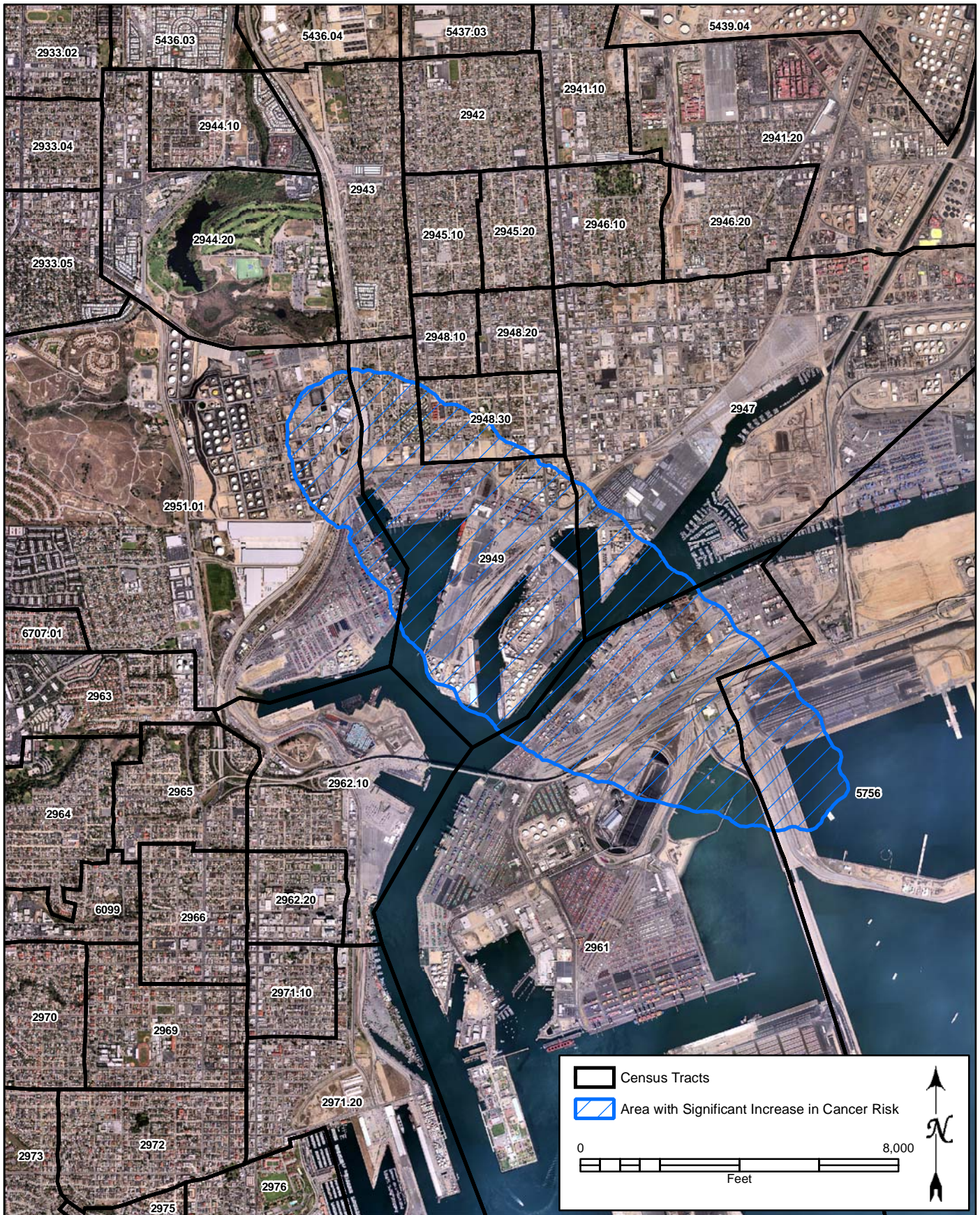
Figure 5-3. Project (with Mitigation) Minus No Federal Action Baseline - Affected Area with Increased Residential Cancer Risk of 10 in a Million Cases or More
