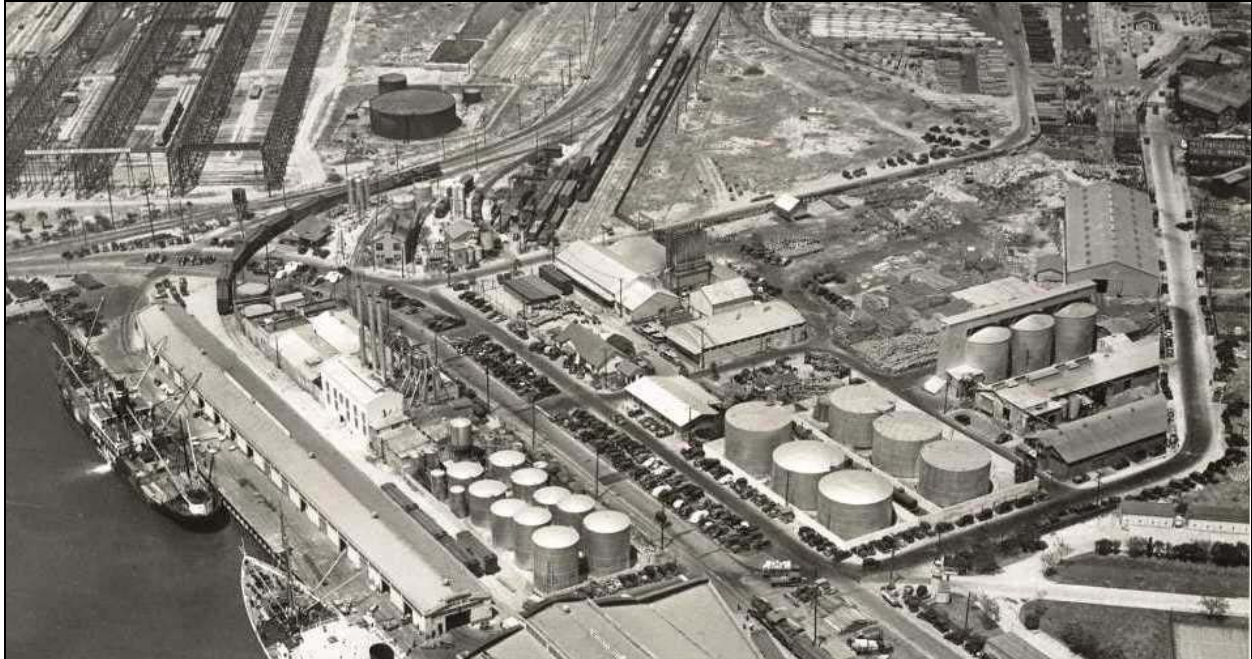
Figure 61 Berth 187 and facilities of the Vegetable Oil Products Company in 1936. From left to right (west to east), the 50-foot-wide, 1,150-foot-long wharf; the 50 by 550 foot umbrella shed; a spur track; the warehouse, refinery, and tank farm; Avalon Boulevard; and the company's copra plant (LAHD Archives, Spence Air Photos, May 12, 1936).
