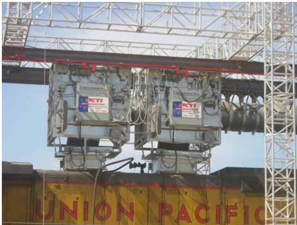
Figure 5. Emissions Intake Bonnets Lowered onto a Locomotive
