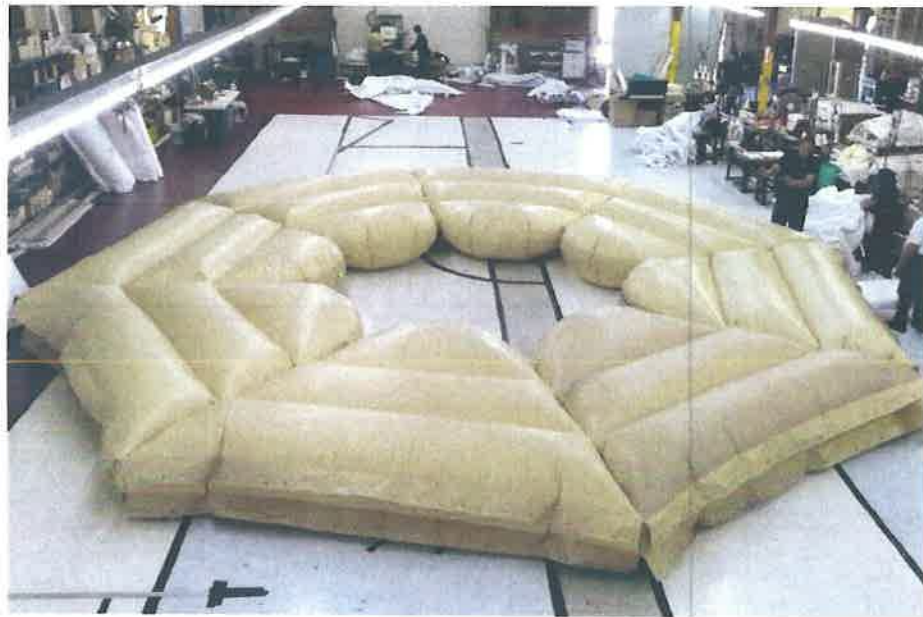
Figure 5. Octagonal Capture Bonnet's Pneumatic Interface Collar
