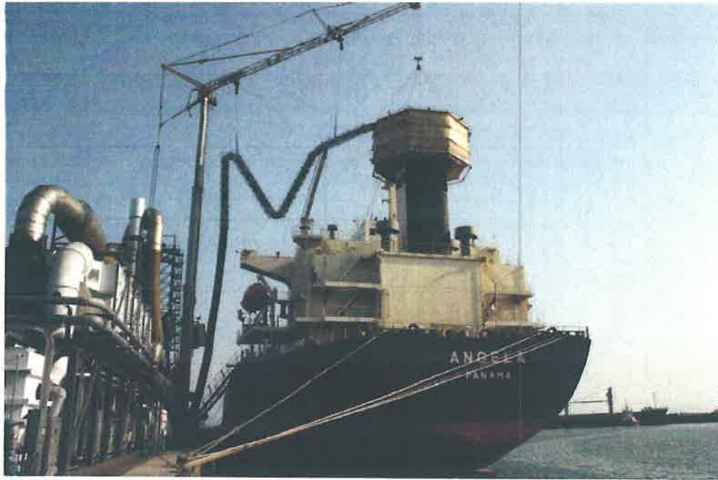
Figure 15. Emission Capture System Attached to the Angela
