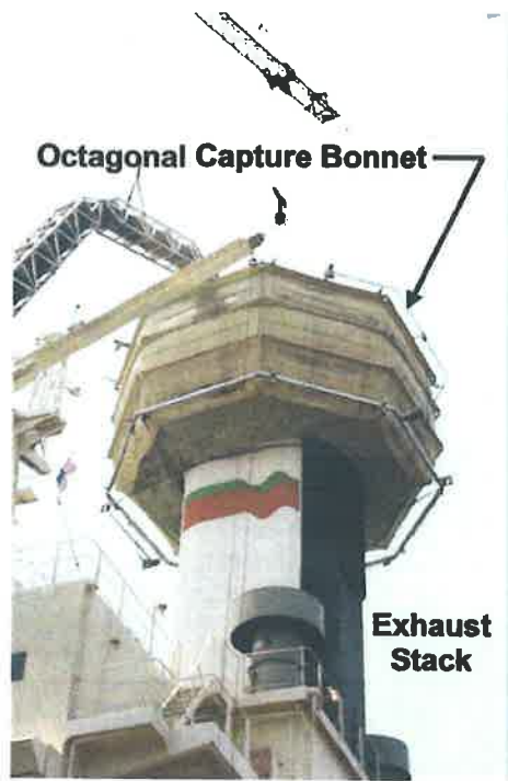
Figure 6. Octagonal Capture Bonnet (attached to the Angela)
