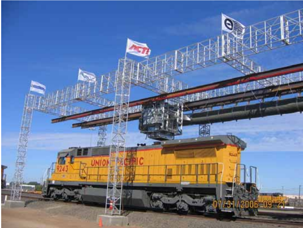
Figure 3. Locomotive under the Exhaust Capture Bonnet
