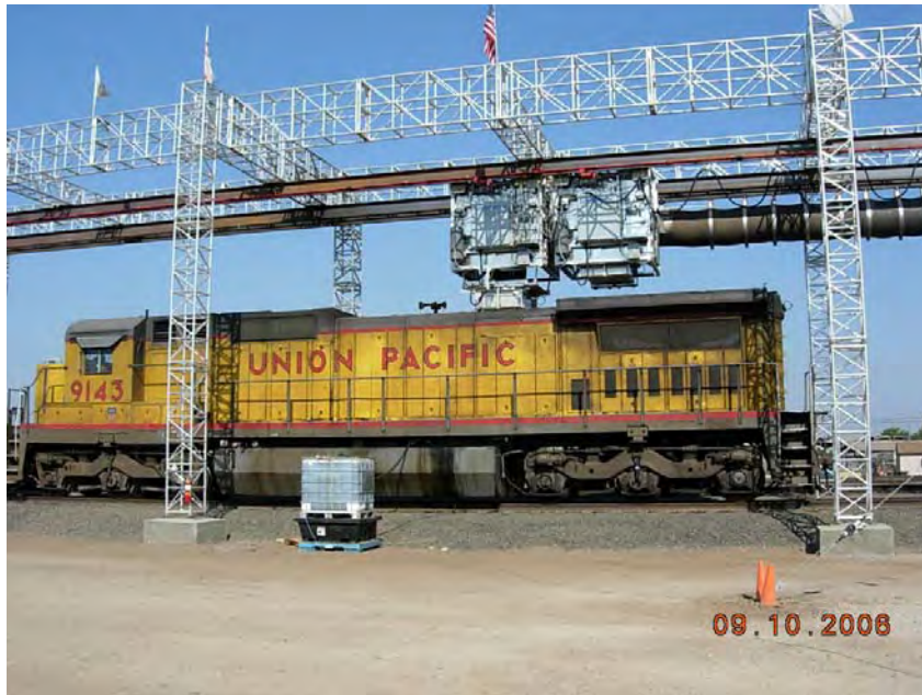
Figure 2: Dash 8 locomotive under emission testing, showing the fuel day tank
