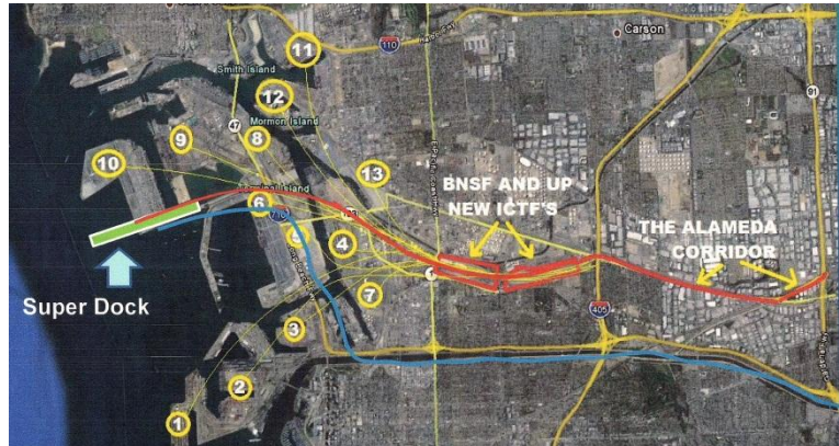
Figure 3 Proposed pipeline (in blue) and Super Dock in relation to existing infrastructure
