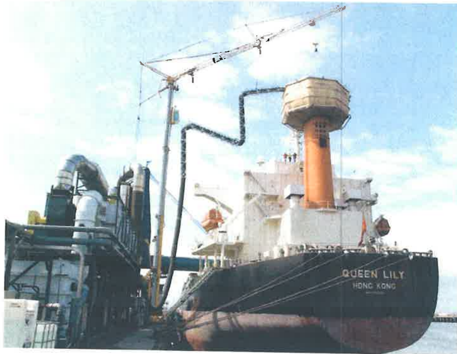
Figure 14. Emission Capture System Attached to the Queen Lily
