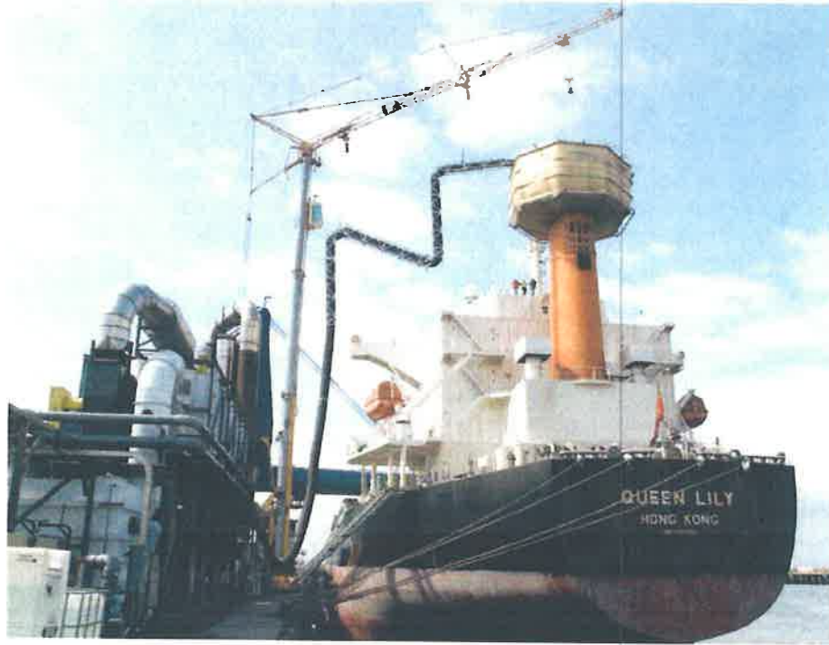
Figure 1. AMECS Attached to the Queen Lily
