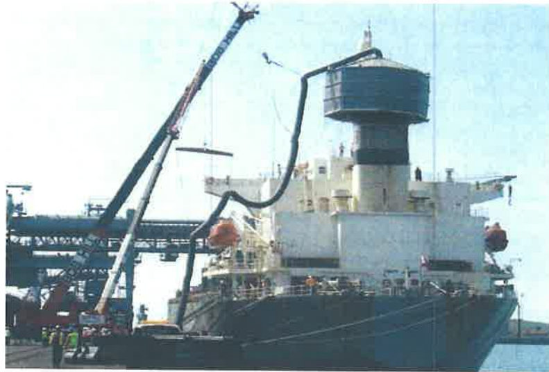
Figure 3. Western Seattle with Octagonal Capture Bonnet
