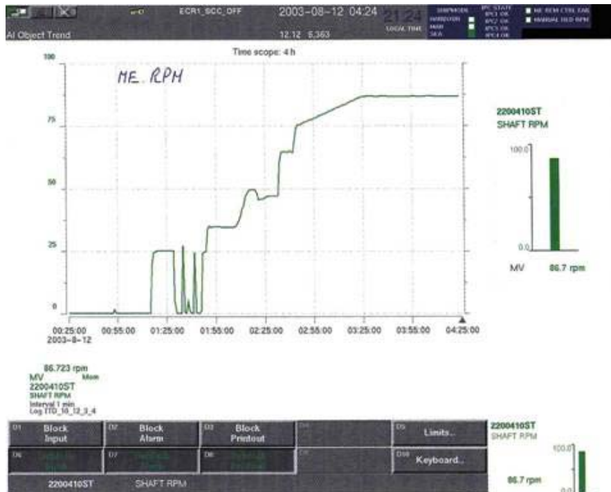
Figure 2.31: Main Engine Speed during Departure, rpm
