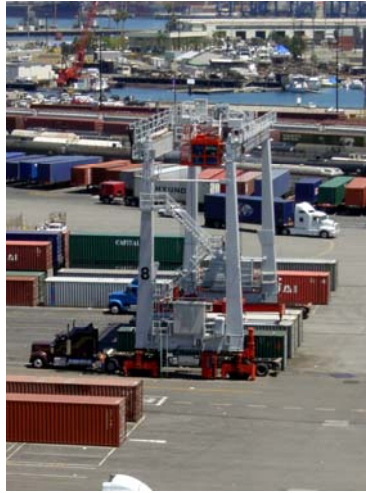
Figure 4.8: Rubber Tired Gantry Crane
