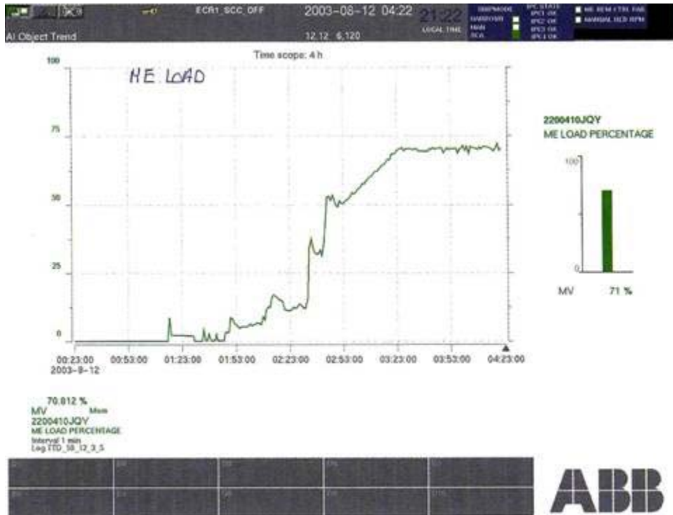
Figure 2.32: Main Engine Load during Departure, %
