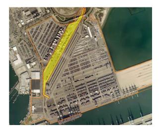
Berths 302-305, On-Dock Railyard Expansion at Fenix Marine Services Container Terminal – An expansion of the existing railyard at Berths 302-305 is in design, which will add five new tracks of approximately 12,000 linear feet. This project will increase the capacity of the existing overall on-dock railyard by about 10%. Total project cost is \$40.5 million with an \$18.1 million federal grant awarded by the United States Maritime Administration (MARAD) and a \$19.2 million federal grant
