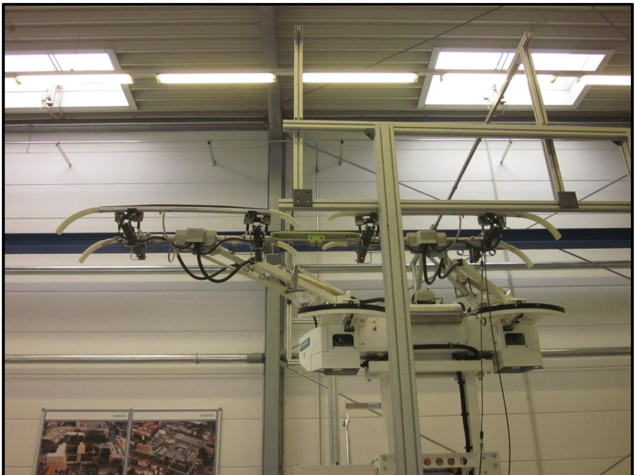
Figure 23 Pantograph horizontal working range test during FAT at Berlin
