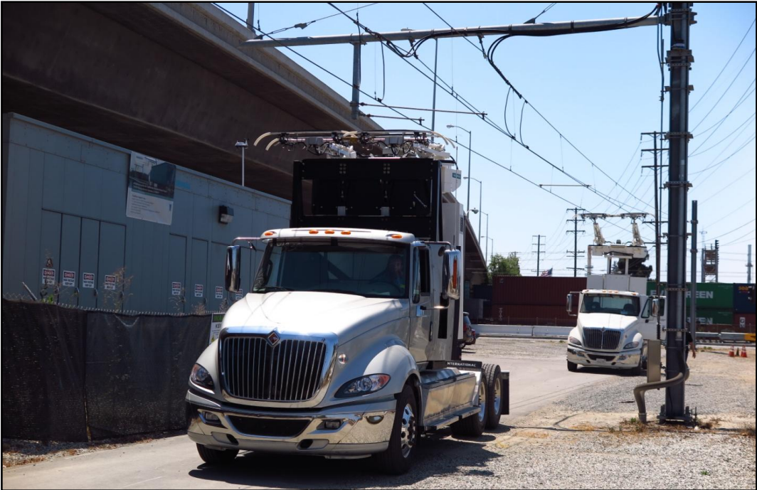
Figure 1 TransPower CCAT (front) and ECAT (behind) at test track next to substation
