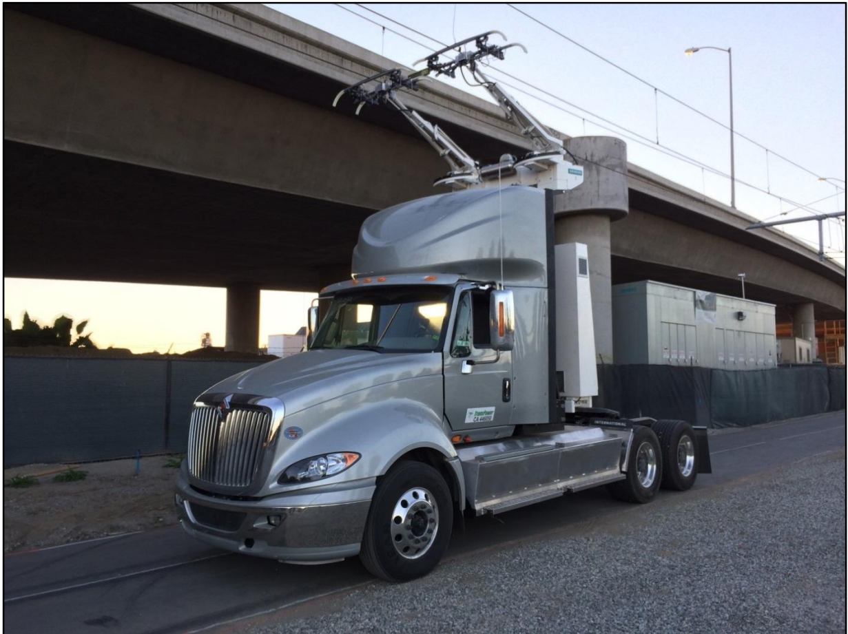
Figure 25 Transpower CNG truck CCAT during site acceptance test
